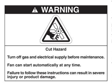
**NOTE 1:** After any maintenance or repair work, always test fire the heater in accordance with the start-up instructions *on Page 19, Section 10 through Page 21, Section 10.3.1* to ensure all safety systems are in working order before leaving the heater to operate. Minor faults may be traced by using the troubleshooting charts *on Page 27, Section 13 through Page 30, Section 13.5.*
